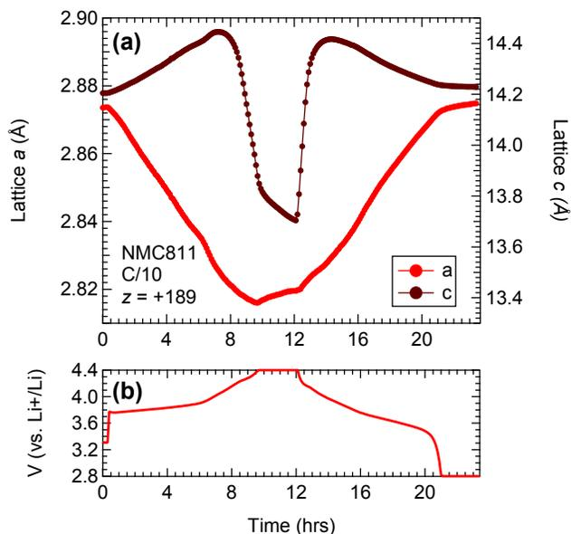
Figure 1. (a) Evolution of *a*- and *c*-lattice parameters during an operando scan at  $z = +189$  microns (relative to center of the film) that exclusively probed the front of an NMC811 electrode. (b) Voltage profile during cycling.
