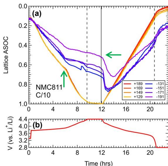
Figure 3. (a) Evolution of accessible state of charge (ASOC) during operando studies of an NMC811 cathode compared for 4 scans at the front of the cathode (purple->blue) and 4 scans at the back of the cathode (red->orange), plotted with (b) the voltage profile during cycling. Dashed and solid lines indicate the end of the CC and CV stages during cycling, respectively.
