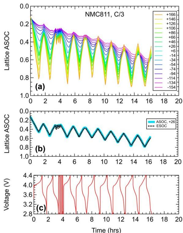
Figure 4. (a) Evolution of the depth-dependent accessible state of charge (ASOC) during *operando* studies of an NMC811 cathode during fast cycling. (b) Comparison of the accessible SOC calculated from diffraction (ASOC) and the electrochemical SOC (ESOC) calculated from the potentiostat which was linearly rescaled and offset to match the ASOC scale. (c) Voltage profile during cycling of this NMC811 film.
